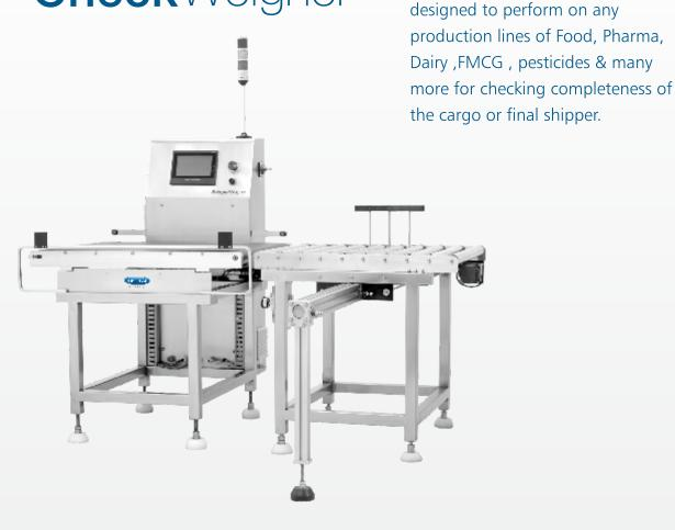
Construction has been made with either SS or Powder coated MS depending upon the environment condition of the application with the core concern of fast & easy cleaning. It is supported by latest automation technology to make it more efficient. The electronics has been placed high above the weighing platform which minimizes the possibilities of inundation of the control panel.
