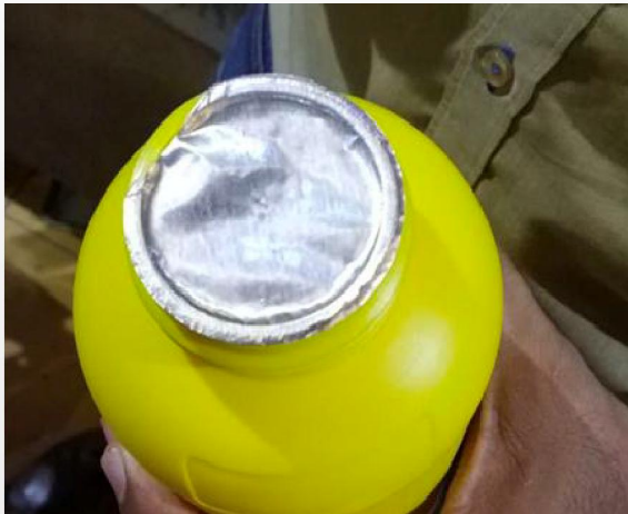
Case 2: PEEL OFF WAD (FLIPPED WAD)
